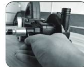
Connect the flexible shaft as shown in the diagram.
