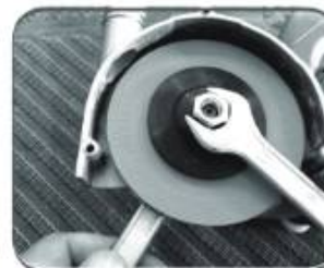
Replace the cutting blade as shown in the diagram for disassembly and installation.
